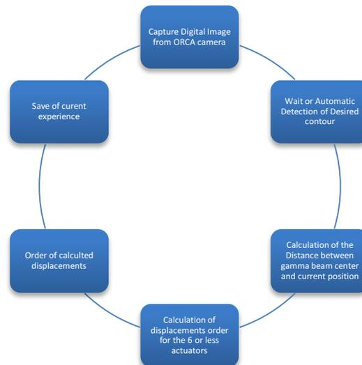
Figure 2 Main workflow diagram of ELICAMM-GAMMA system
