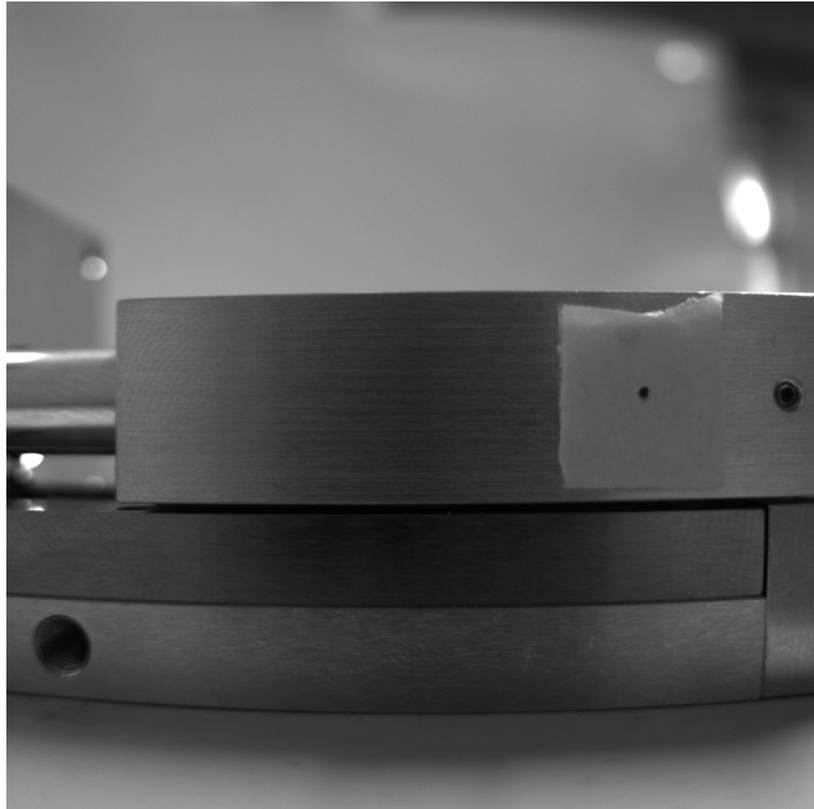
*Figure 4 Sliding sleeve of the actuator with a reference point used for testing the repetitive movement that illustrate the accuracy in positioning of sample holder based on firmware developed. (represent achievement of a component test for alignment system)*
