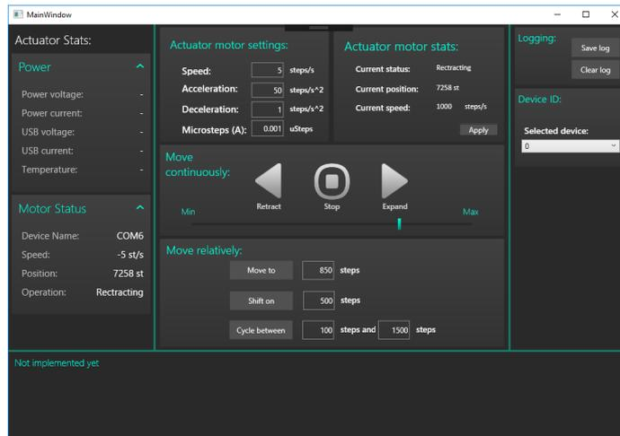
Figure 3 Acting system interface for manual positioning of the sample holder inside the interaction chamber
