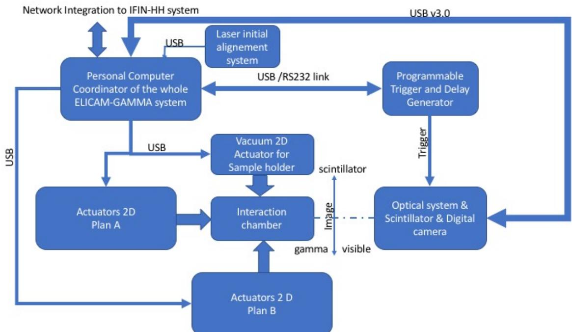
Figure 1 Block diagram of ELICAM-GAMMA system
