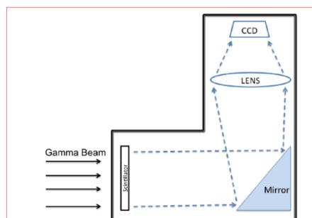
Figure 5 Principle of the alignment with CCD
