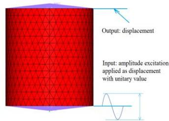
**Fig. 1.** Physical model of the inertial damper      **Fig. 2.** Finite element model of the damper
