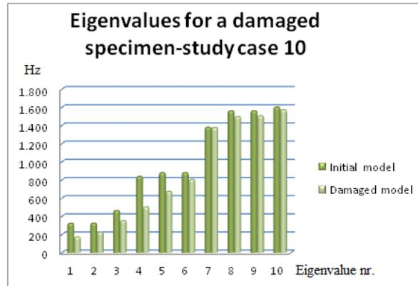
**Fig. 5.** The first 10 eigenvalues for the scenario nr. 10 (initial and damaged model)
