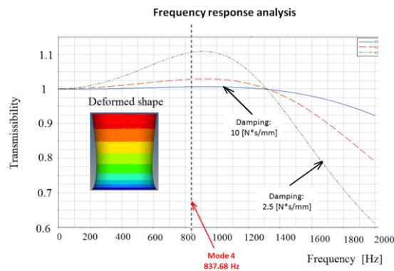
**Fig. 4.** Frequency response for an inertial damper with steel balls
