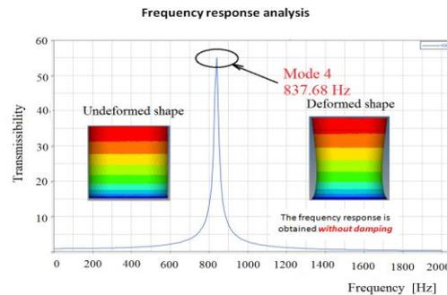
**Fig. 3.** Frequency response for a rubber model
